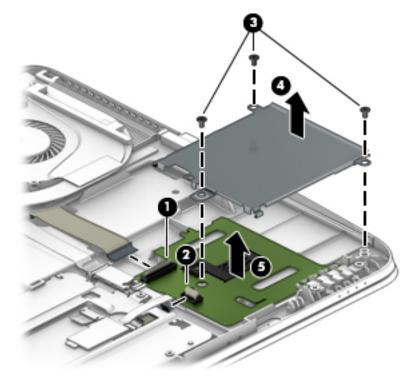
Reverse this procedure to install the smart card reader board.
