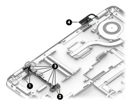
6. Remove the 4 Phillips M2.5×5.0 screws (1) from the display hinges.
