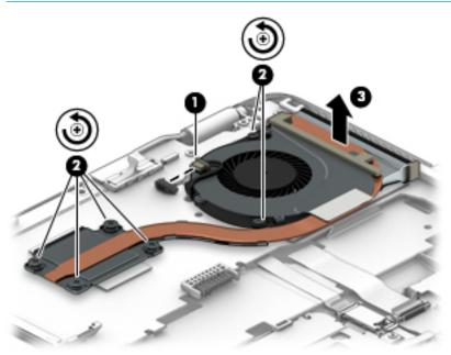
The thermal material must be thoroughly cleaned from the surfaces of the heat sink and the system board components each time the heat sink is removed. Replacement thermal material is included with the heat sink, processor, and system board spare part kits.
