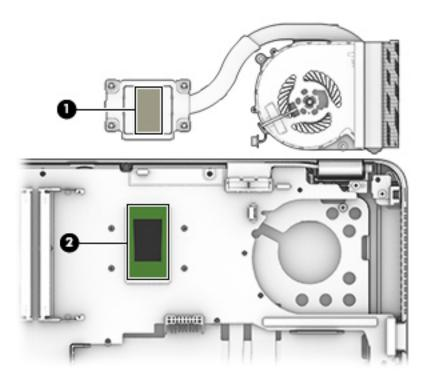
Reverse this procedure to install the heat sink/fan assembly.
