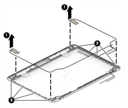
The WLAN antennas are spared with the display enclosure.
