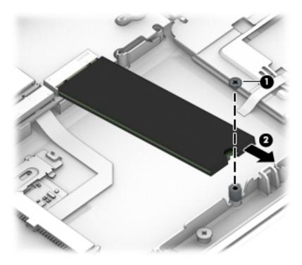
Remove the drive (2) by pulling it away from the connector. 2.
