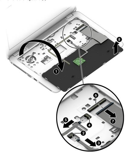
Reverse this procedure to install the keyboard.
