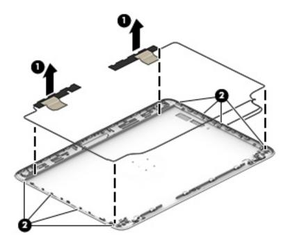
The WWAN antennas are spared with the display enclosure.
