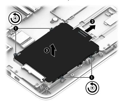
To remove the hard drive cover from the hard drive, remove the 4 Phillips M3.0×3.0 screws (1) that secure the bracket to the drive, and then lift the bracket up and off the hard drive (2).
