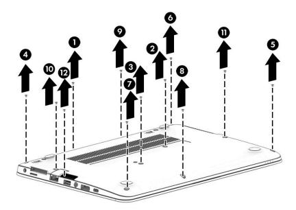
5. Pry up on the top (near the display hinge) of the bottom cover to disengage it from the computer.
