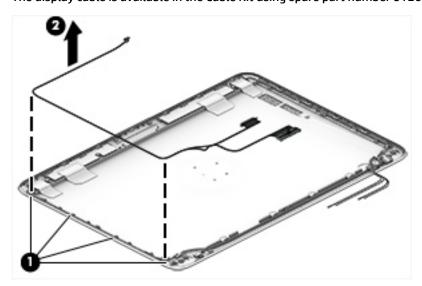
**16.** If it is necessary to replace the WLAN antennas, peel the transceivers off the top of the display enclosure **(1)**, and then remove the antennas from the routing paths on the side of the display enclosure **(2)**.
