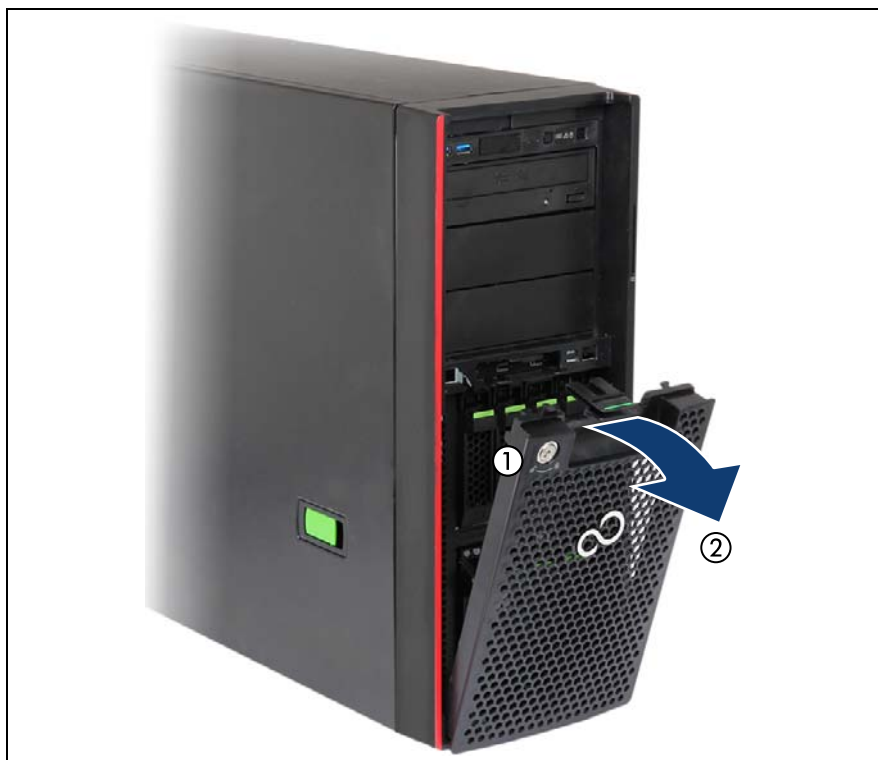
Figure 8: Removing the HDD cover
