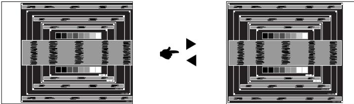
2) Stretch the right side of the picture frame to the right edge of the display area by adjusting the Clock Frequency.
