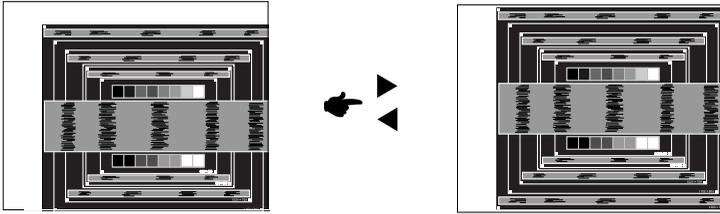
⑥ 1) Adjust the H-Position so that the left side of the picture frame will move to the left edge of the display area.
