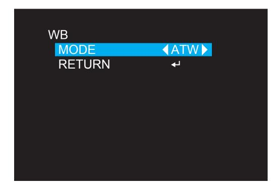
**ATW (Automatic White Balance):** The camera sets the White Balance automatically according to the surrounding lighting conditions so that the most natural reproduction of color tone can be obtained in the image. We recommend you use this setting in most circumstances.
