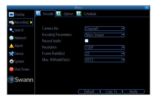
**Record Audio:** If you have a microphone or some other audio device connected to the DVR's audio input, click the checkbox to record audio.
