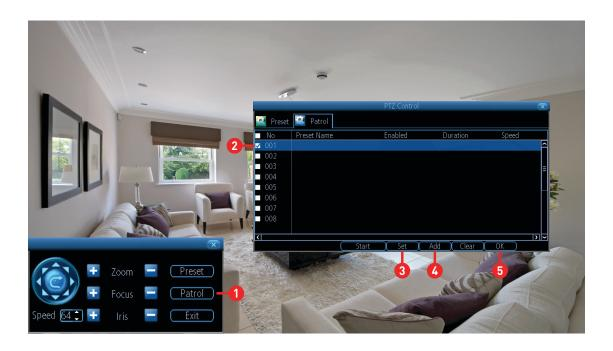
Patrol mode instructs the DVR to automatically move the camera according to the Preset positions that have been created.
