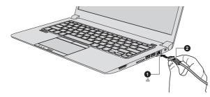
Figure 4-8 Connecting the LAN cable (Z30-C)
