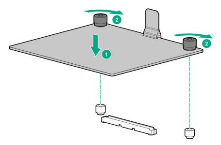
• For Type-p Smart Array controllers, install the controller into an expansion slot.
