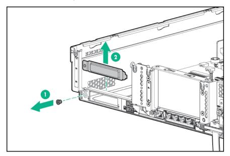
Install the FlexibleLOM adapter:
