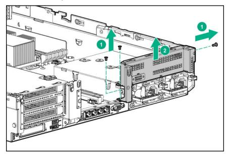
Install the drive cage compatible rear wall.
