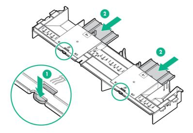
**b.** Install the appropriate retention clip onto the air baffle.
