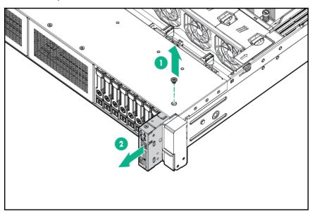
Route the cable through the opening in the front of the server, and then install the SID power switch module. Secure the module using the existing screw.
