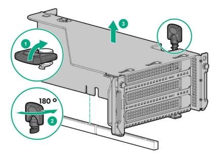
Identify and then remove the PCIe blank from the riser cage.
