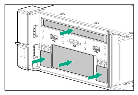
• If a 2SFF drive cage is installed, then install the airflow labels as shown.
