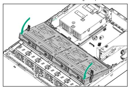
**13.** Connect the power and data cables to the drive backplane.
