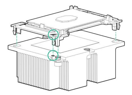
11. Install the processor heatsink assembly.
