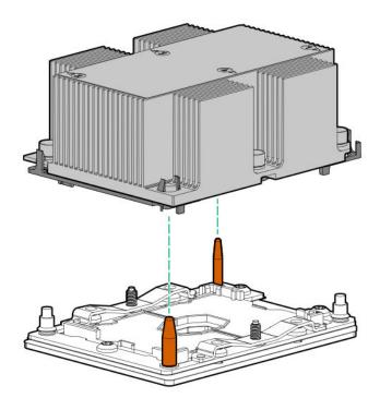
**d.** Using a T-30 Torx screwdriver, tighten the nuts until they stop.
