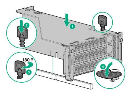
To install the riser in the secondary position, install the secondary riser cage.
