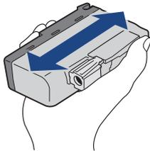
4. Insert the ink cartridge in the direction of the arrow on the label.
