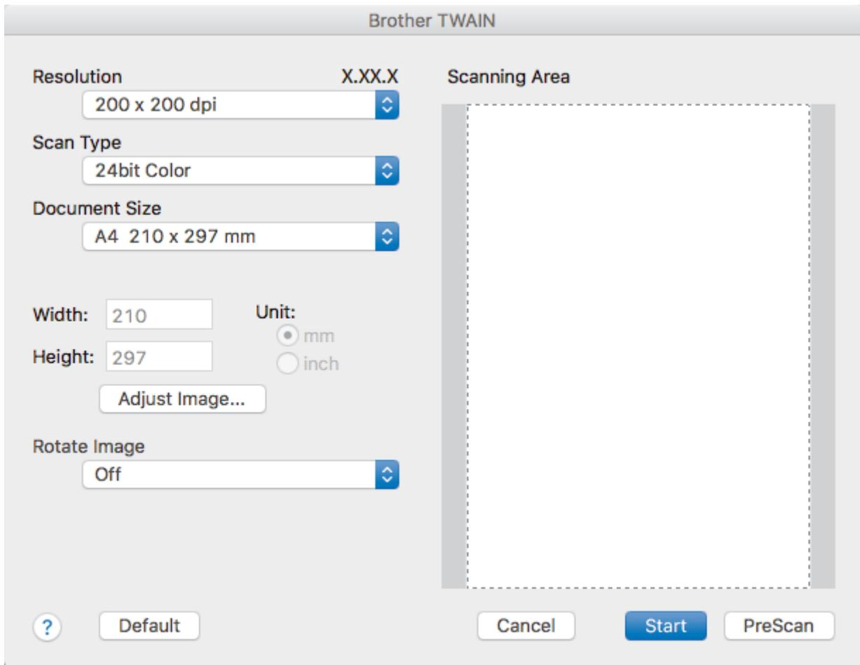
2. Change the scan settings, such as **Resolution**, **Scan Type**, or **Adjust Image**, if needed.
