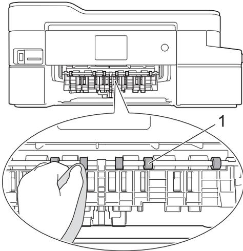
5. Lift the Jam Clear Flap (2), and then clean the back side of the Paper Feed Rollers (1) with a soft lint-free cloth moistened with water. After cleaning, wipe the rollers with a dry, soft lint-free cloth to remove all moisture.
