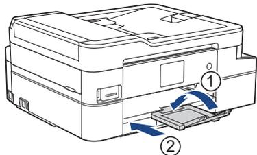
3. Pull the paper tray completely out of the machine.
