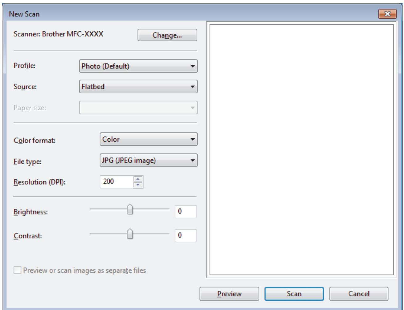
6. Adjust the settings in the Scanner Setup dialog box, if needed.
