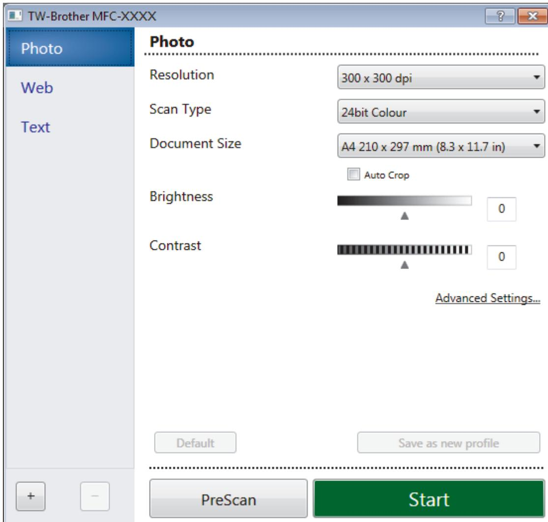
8. Adjust the settings in the Scanner Setup dialog box, if needed.
