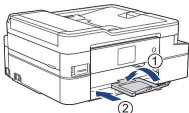
2. Pull the paper tray completely out of the machine.
