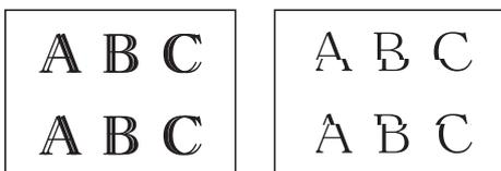
After the print alignment is adjusted correctly, text looks like this.
