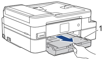
3. Clean the Base Pad (1) with a soft lint-free cloth moistened with water. After cleaning, wipe the pad with a dry, soft lint-free cloth to remove all moisture.
