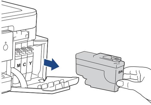
3. Open the new ink cartridge bag for the colour indicated on the LCD, and take out the ink cartridge.
