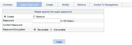
Note: Use the super password to switch from the current user level to the management level.
