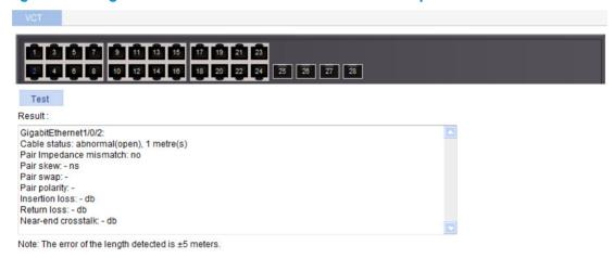
The result displays the cable status and length. The cable status can be normal, abnormal, abnormal (open), abnormal (short), or failure.
