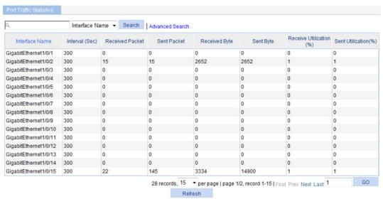
When the bandwidth utilization is lower than 1%, 1% is displayed.
