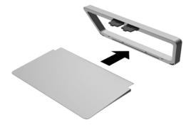
3. Lift up the bottom of the display panel (1) and insert the stand into the slot on the back of the display panel until it clicks in place (2).
