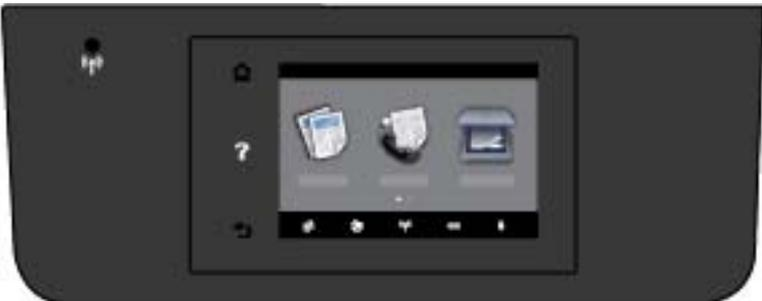
A photograph of the printer's control panel. The wireless light indicator, located at the top left, is not illuminated. The central touchscreen displays a menu with three printer icons and a question mark icon on the left. | <p data-bbox="1023 254 1445 296">The wireless capability of the printer is turned off.</p>                                              |
