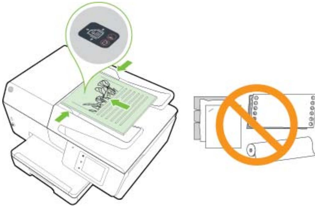
2. Slide the paper-width guides inward until they stop at the left and right edges of the paper.
