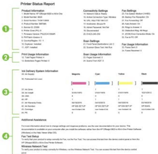
1. **Product Information:** Shows printer information (such as the printer name, model number, serial number, and firmware version number), and the accessories that are installed (such as the automatic two-sided printing accessory or duplexer).
