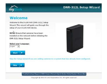
Note: The computer used to access the NVR must be on the same subnet as the NVR. If your network is using a DHCP server, the NVR will automatically be in the same subnet.
