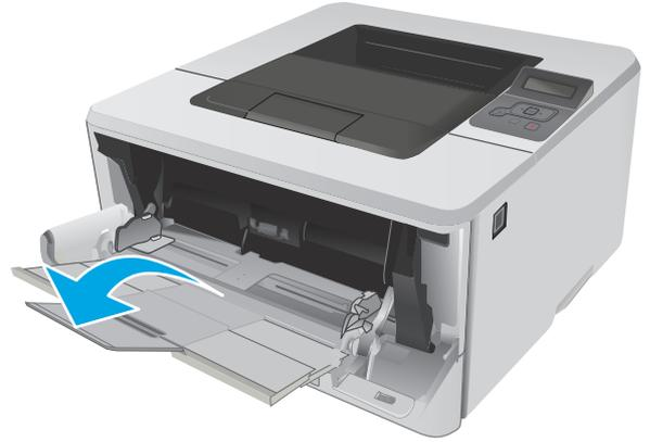
4. Press down on the tab on the right paper guide, and then spread the paper guides to the correct size.
