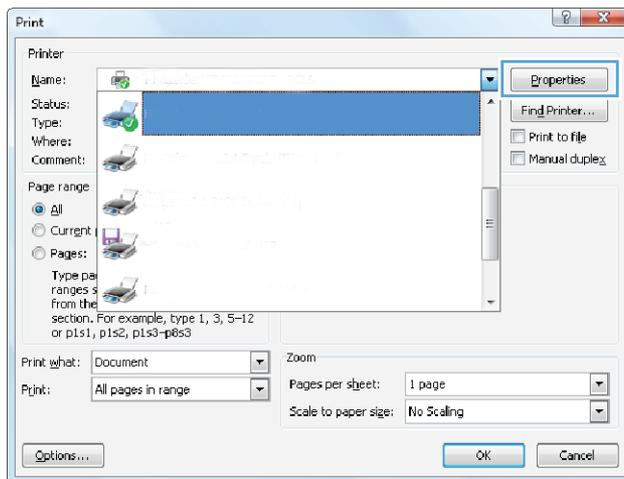
3. Click or tap the tabs in the print driver to configure the available options. For example, set the paper orientation on the **Finishing** tab, and set the paper source, paper type, paper size, and quality settings on the **Paper/Quality** tab.
