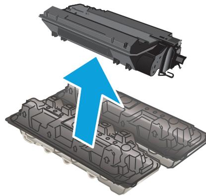
6. Align the toner cartridge with the tracks inside the printer, and install the toner cartridge until it is firmly seated.
