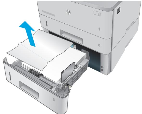
3. Verify that the rear paper guide is adjusted to the indentation for the correct paper size. If necessary, pinch the release and move the rear paper guide to the correct position. It should click into place.
