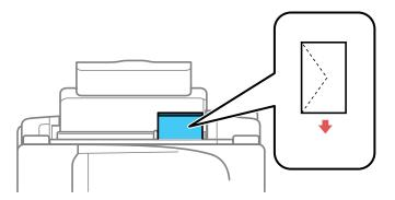
• Load a sheet of loose-leaf or other paper with holes facing as shown.
