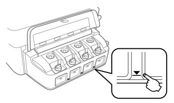
**Note:** The product has a low ink alert system. The accuracy of this system depends on the user refilling the ink tanks correctly. The product cannot directly measure the ink levels in the tanks; instead it estimates the amount of ink remaining by internally monitoring ink usage. The low ink alert system may generate inaccurate messages if the ink tanks are not refilled according to these instructions.
