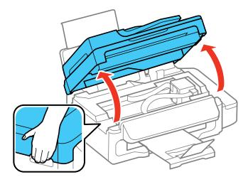
**Caution:** Do not touch the flat white cable inside the printer. Do not lift the scanner unit while the document cover is open.
