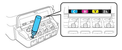
5. Snap off the tip of the bottle cap, but do not dispose of it so you can use it to seal the bottle cap later, if necessary. Then remove the bottle cap and carefully remove the protective seal (avoid touching the ink underneath the seal). Close the bottle cap tightly.
