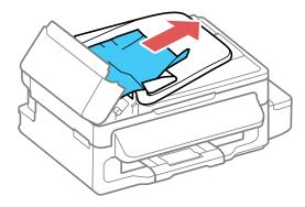
**Caution:** Do not remove paper jammed inside the ADF without opening the cover or you could damage the ADF.
