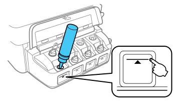
7. If any ink remains in the ink bottle after filling the ink tank, place the bottle cap tip securely on the bottle cap and store the ink bottle upright for later use.
