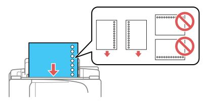
6. Slide the edge guide against the paper, but not too tightly. Then, flip the feeder guard back.
