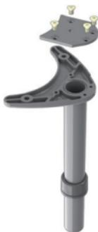
4. Use a Phillips screwdriver to remove the screw and two washers shown, and disconnect the threaded shaft from the base of the desk clamp **(3)**. Slide the plate back onto the shaft.
