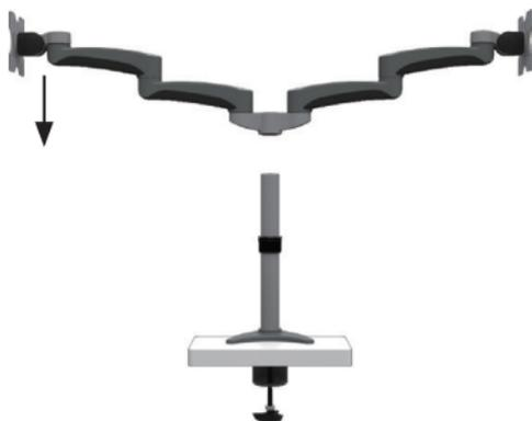
8. Place the dual mount **(2)** and the attached LCD arms **(1)** attached onto the pole.
