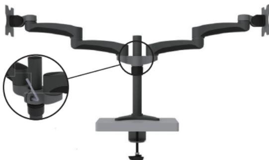
9. Use the M5 Allen key **(9)** to tighten the dual mount **(2)**.
