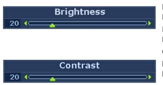
Press the key to display the Brightness and Contrast indicators. Further press the or keys, then the ENTER key to select Brightness or Contrast. The key will increase the level, while the key will decrease the level.
