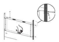
4. Secure the front cover of the device box (F) to the later with the included flat head screws (M3xL8) (C) by a Phillips screwdriver.
