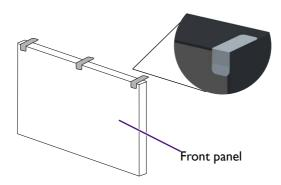
4. After the displays are mounted and fastened, check if the space between each display is just enough for removing the gap inspection pad smoothly. If the pad is trapped, adjust the screws to release more space.
