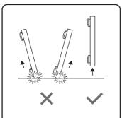
Be careful not to scratch any parts of the display when upturning the display.
