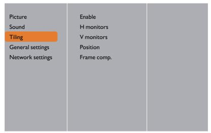
With this function you can create a single large-screen matrix (video wall) that consists of up to 225 sets of this display (up to 15-sets on the vertical and 15-sets on the horizontal sides).
