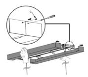
5. Remove the spring washer and nut from the expansion screw and secure the bracket (A) to the ceiling.
