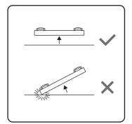
Lift the display up horizontally by holding the four (4) handles. Do not lift the display against its corner.
