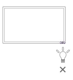
When using the remote control, make sure the display's remote control sensor window is NOT exposed to direct sunlight or strong reflected light, e.g. tile flooring.
