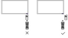
When using the remote control, confirm there is no object between the remote control and the remote sensor of the product.
