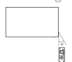
For IL430/ IL490/ IL550, when two displays place together, the signal of the remote control is easily interfered by the Touch screen signal.
