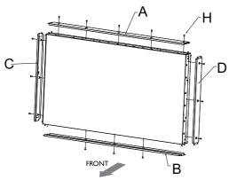
2. On each corner, mount a corner enclosure piece and fasten each one with 4 of the 5mm M3 screws.
