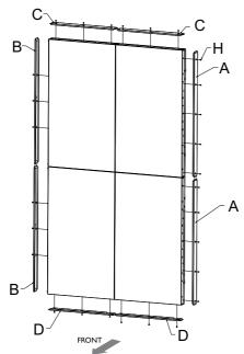
On each corner, mount a corner enclosure piece and fasten each one with 4 of the 5mm M3 screws. Where the displays meet, use a flat enclosure piece, and fasten each of these too with 4 of the 5mm M3 screws.
