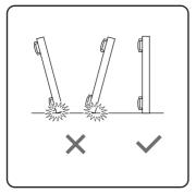
When you want to upturn the display, stand the display vertically to make sure its weight spread evenly on the surface.
