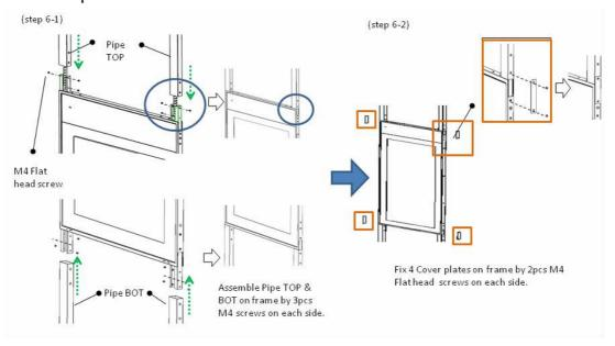
Step 7: Mounting Pipe TOP and Pipe BOT with ceiling and ground
