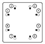
There are two loops of screw holes (outer & inner), depend on the design of each model. (Please check the user manual for using loop information)
