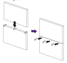
5. Insert the pad again and swipe the pad horizontally and vertically between the gap to ensure it can move smoothly. Ignore the black tapes on the edge if they stop you. Refer to Recommended gap between displays on page 23 for the minimum distance required for each model.
