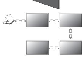
3. Set the horizontal and vertical position of the display wall matrix. This helps your computer identify how many displays are connected and how to display the image. See Setting the display position on page 31 for more information.
