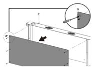
2. Secure the display box (F) to the display with the included flat head screws (M3xL8) (C) by a Phillips screwdriver.
