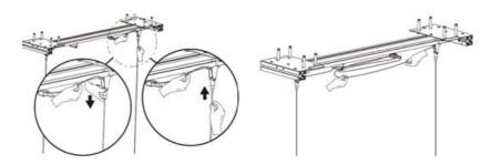
2. Replace the plastic covers to the left and right of the bracket before securing them with the included flat head screws (M3xL8) (C) by a Phillips screwdriver.
