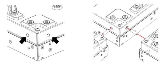
There are 8 holes on the four corners of displays designed for plug-in the edge alignment pin.
