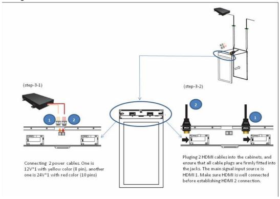
Step 4: Fixing the double sided display with Frame
