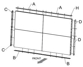
On each corner, mount a corner enclosure piece and fasten each one with 4 of the 5mm M3 screws. Where the displays meet, use a flat enclosure piece, and fasten each of these too with 4 of the 5mm M3 screws.
