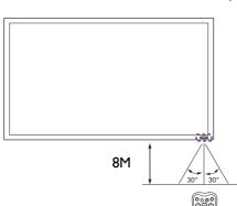
Operate the remote control from a location closer to the display's remote control sensor window. Adjust the distance between the remote control and the display.
