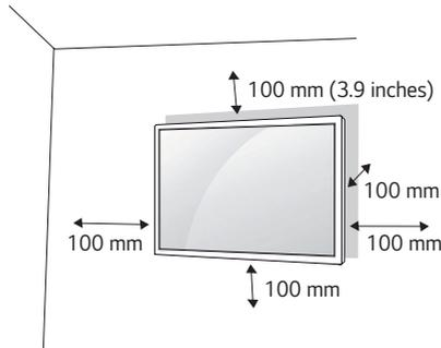
To install your monitor on a wall, attach a wall mounting bracket (optional part) to the back of the monitor. Make sure that the wall mounting bracket is securely attached to the monitor and to the wall.
