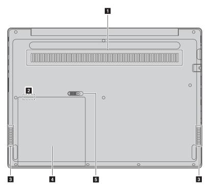
1 Ventilation slots Dissipate internal heat.
