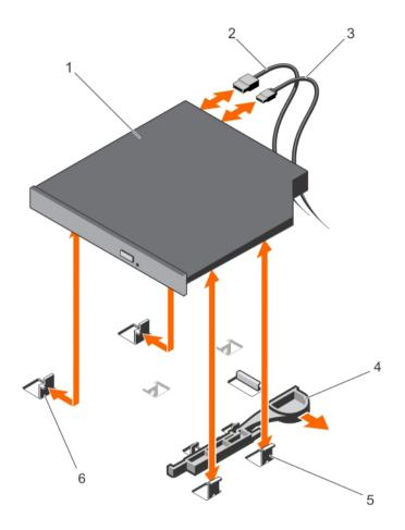
Figure 27. Removing and installing the standard optical drive
