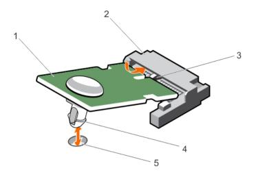
Figure 57. Installing the TPM
