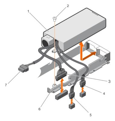
Figure 41. Removing and installing a non-redundant power supply
