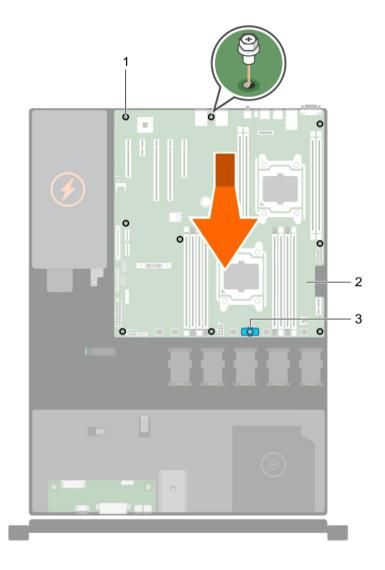
Figure 56. Removing and installing the system board
