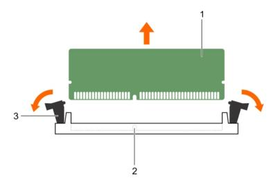
Figure 17. Removing memory module
