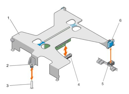
Figure 30. Removing and installing the expansion-card riser
