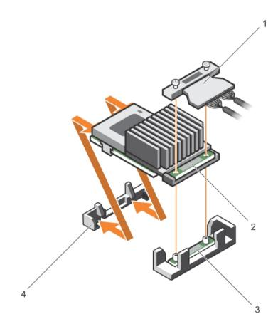
Figure 35. Removing and installing the integrated storage controller card
