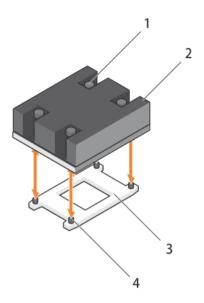
Figure 36. Removing and installing a processor heat sink
