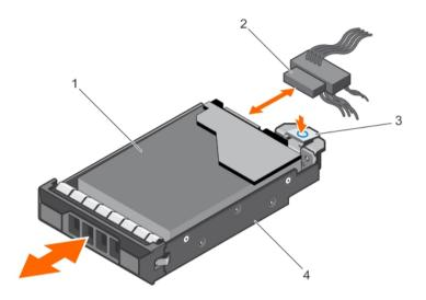
Figure 21. Removing and installing a cabled hard drive
