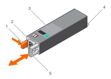
Figure 40. Removing and installing a redundant power supply
