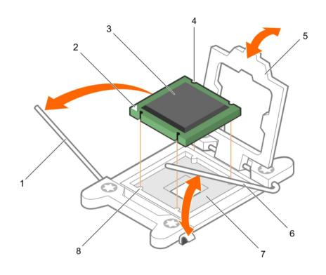
Figure 38. Removing and installing a processor
