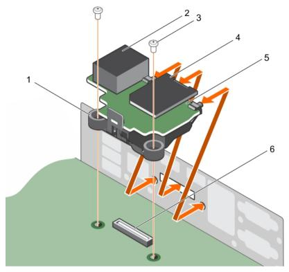
Figure 32. Removing and Installing the iDRAC port card
