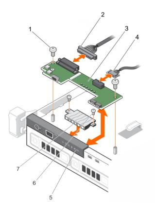
Figure 52. Removing and installing the control-panel module—four cabled hard-drive chassis
