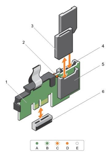
Figure 34. Removing and installing the Internal Dual SD Module (IDSDM)
