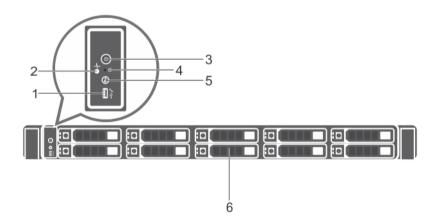
Figure 3. Front-panel features and indicators—ten 2.5 inch hot-swappable hard-drives/SSDs chassis
