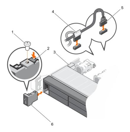
Figure 51. Removing and installing the control panel—ten 2.5 inch hard-drives/SSDs chassis
