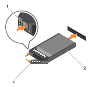
Figure 22. Removing and installing a hot-swap hard drive
