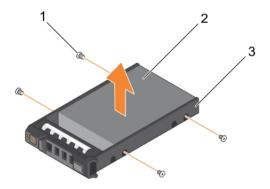
Figure 25. Removing and installing a hard drive into a hard-drive carrier
