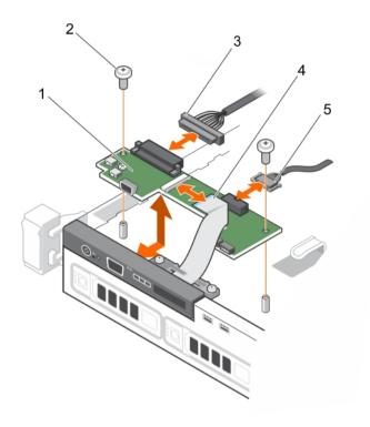
Figure 53. Removing and installing the control panel module—four hard-drive chassis
