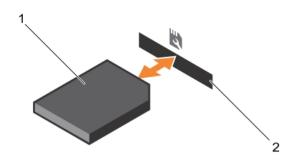
Figure 33. Removing and installing the SD vFlash media card
