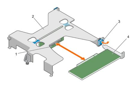
Figure 31. Removing and installing the expansion card from expansion-card riser
