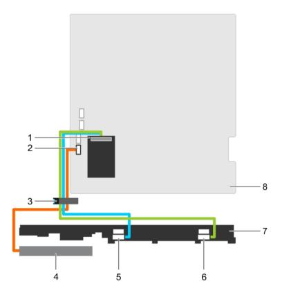
Figure 46. Cabling diagram—2.5 inch (x8) SAS/SATA backplane
