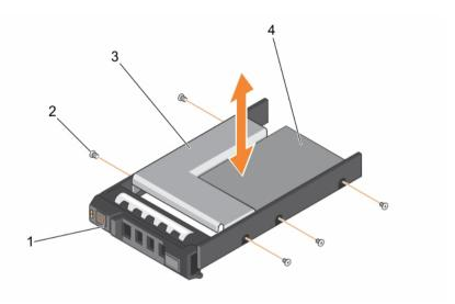
Figure 24. Removing and installing a hard-drive adapter into a 3.5 inch hard-drive carrier
