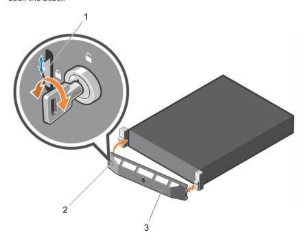
Figure 12. Removing and installing the front bezel
