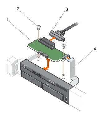
Figure 54. Removing and Installing the control panel module—eight hard-drive chassis
