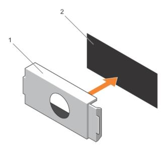
Figure 42. Removing and installing the power supply blank
