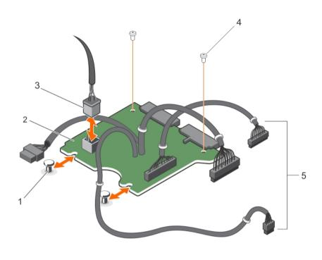
Figure 55. Removing and installing the power interposer board
