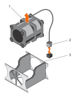
Figure 28. Removing and installing a cooling fan
