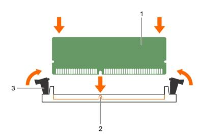
Figure 18. Installing the memory module
