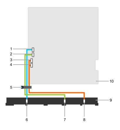
Figure 48. Cabling diagram—2.5 inch (x10) SAS/SATA backplane
