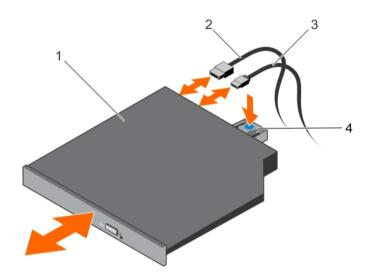
Figure 26. Removing and installing an ultra slim optical drive
