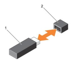
Figure 29. Replacing the internal USB key
