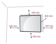
Install the monitor at least 100 mm away from the wall and leave about 200 mm of space at each side of the monitor to ensure sufficient ventilation.
