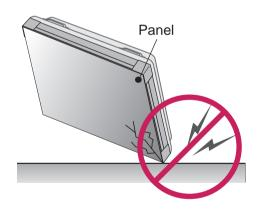
If the product is tilted onto the edge of the panel, the panel may be damaged.
