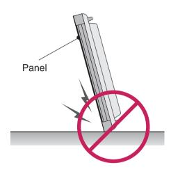
If the product is tilted onto the bezel, the bottom of the panel may be damaged.
