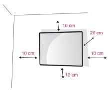
Ilnstall the monitor at least 10 cm away from the wall and leave about 20 cm of space at each side of the monitor to ensure sufficient ventilation.
