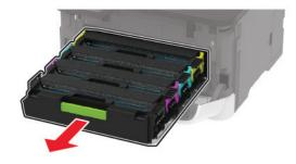
**5** To avoid stray toner contamination, place a sheet of paper on the top of the print cartridge tray, and then insert the print cartridge tray.
