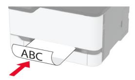
• Load envelope with the flap side down and against the right side of the paper guide.
