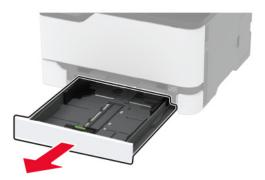
Remove the used manual feeder.
