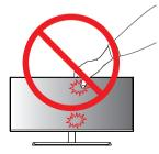
If you use the monitor panel without the stand base, its joystick button may cause the monitor to become unstable and fall, resulting in damage to the monitor or human injury. In addition, this may cause the joystick button to malfunction.
