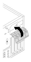
Figure 24. Closing the PCIe card latch
