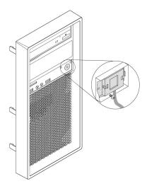
Figure 11. Removing the power button
