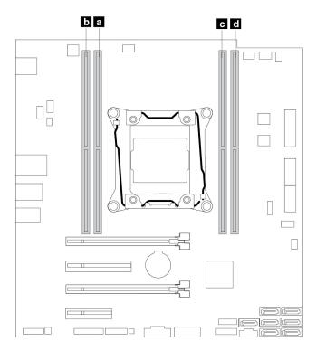
Figure 25. Memory module installation order
