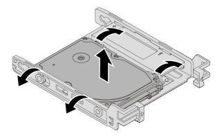
Figure 64. Removing the 2.5-inch storage drive from the bracket
