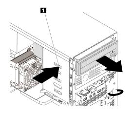
Figure 29. Removing the optical drive
