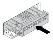
Figure 47. Installing the plastic bracket with the 2.5-inch storage drive into the front-access storage enclosure
