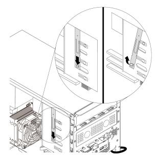
Figure 30. Removing the optical-drive retainer from the computer
