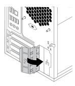
Figure 17. Closing the PCIe card latch
