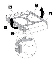
Figure 79. Installing the storage drive into the bracket
