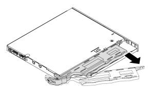
Figure 49. Removing the bracket from the slim optical drive
