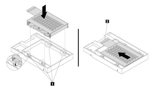
Figure 45. Installing the adapter into the converter
