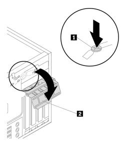
Figure 18. Opening the PCIe card latch
