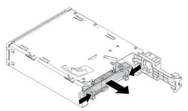
Figure 53. Removing the conversion bracket from the kit
