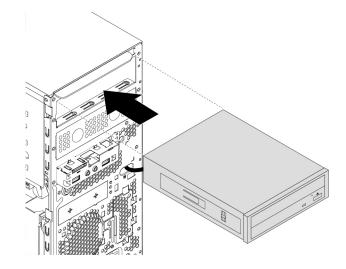
Figure 32. Installing the optical drive
