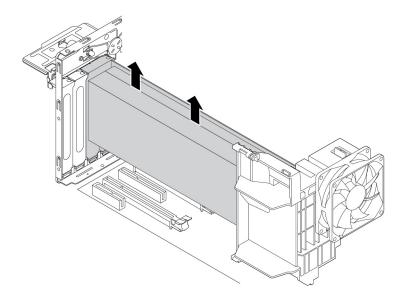
Figure 21. Removing the full-length PCIe card
