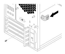
Figure 75. Installing the cover presence switch
