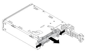
Figure 63. Removing the 2.5-inch storage drive from the kit
