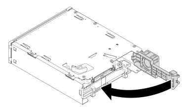
Figure 61. Pivoting the rear cover inward
