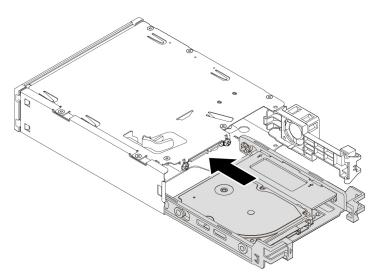
Figure 70. Installing the new 2.5-inch storage drive with bracket into the kit
