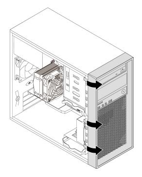
Figure 10. Removing the front bezel
