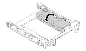
Figure 57. Unfolding the bracket
