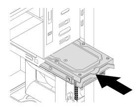
Figure 80. Installing the primary storage drive
