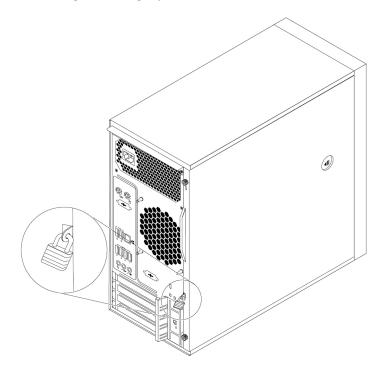
Figure 7. Installing a padlock
