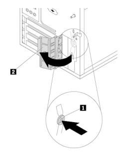
Figure 13. Opening the PCIe card latch
