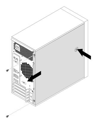
Figure 9. Removing the computer cover
