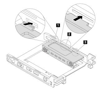
Figure 68. Inserting the tabs into the corresponding slots
