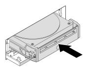
Figure 38. Installing the 3.5-inch storage drive into the front-access storage enclosure
