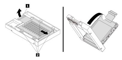
Figure 42. Removing the adapter from the converter
