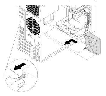
Figure 91. Installing the rear fan assembly
