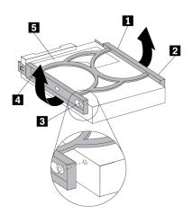
Figure 82. Installing the storage drive into the bracket
