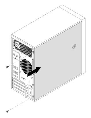
Figure 92. Reinstalling the computer cover
