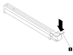
Figure 19. Disengaging the retaining latch
