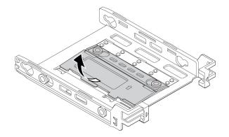
Figure 67. Folding the bracket
