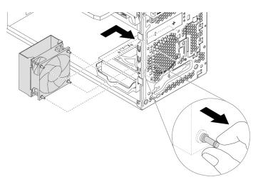
Figure 89. Installing the front fan assembly
