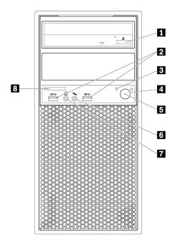
Figure 1. Front connectors, controls, and indicators
