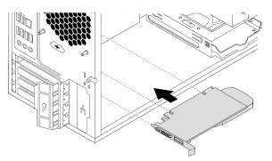
Figure 16. Installing a PCIe card
