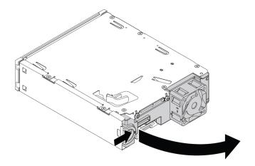
Figure 52. Opening the rear cover of the kit
