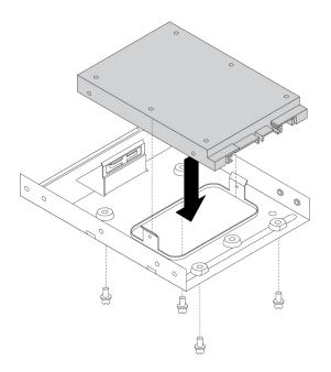
Figure 86. Installing a new 2.5-inch storage drive into the storage-drive converter
