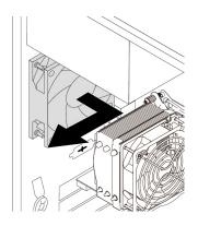
Figure 90. Removing the rear fan assembly
