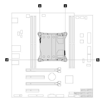
Figure 77. Removing the heat-sink-and-fan assembly
