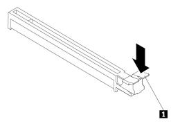
Figure 14. Disengaging the retaining latch
