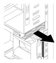
Figure 78. Removing the primary storage drive
