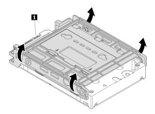
Figure 54. Removing the storage drive from the bracket
