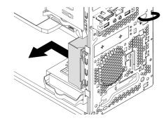
Figure 88. Removing the front fan assembly
