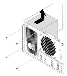
Figure 76. Removing the screws for the power supply assembly
