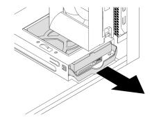
Figure 81. Removing the secondary storage drive
