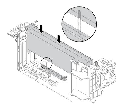
Figure 22. Installing a full-length PCIe card
