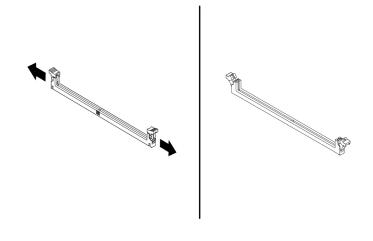
Figure 27. Opening the retaining clips
