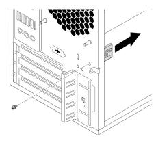
Figure 74. Removing the cover presence switch
