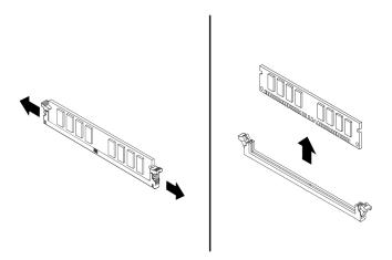
Figure 26. Removing a memory module
