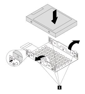
Figure 44. Installing the storage drive into the adapter
