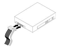
Figure 33. Connecting the cables to the rear of the new optical drive
