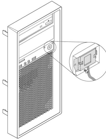
Figure 11. Removing the power button
