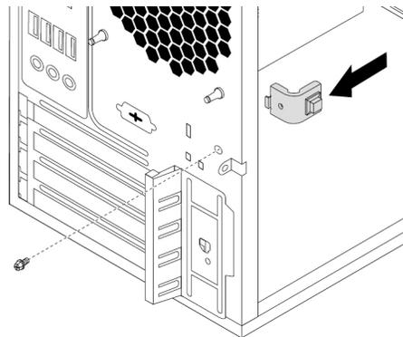
Figure 75. Installing the cover presence switch
