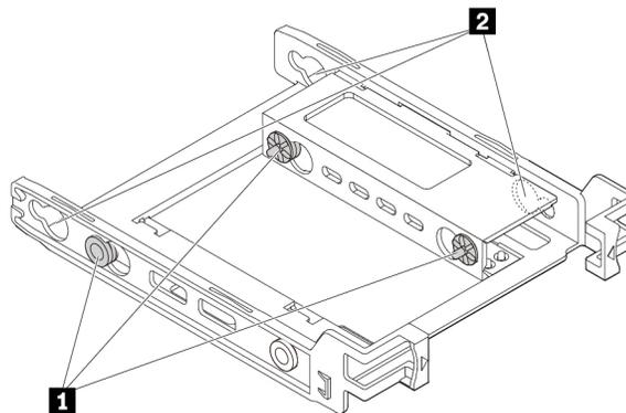
Figure 55. Removing pins and installing them into slots
