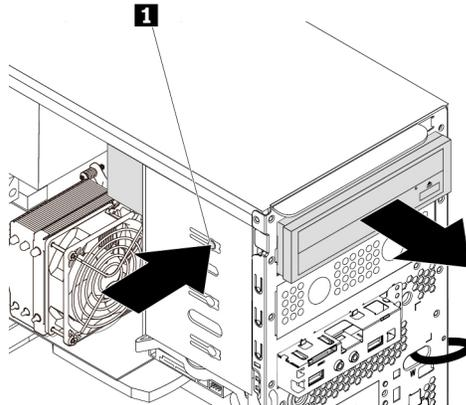
Figure 29. Removing the optical drive
