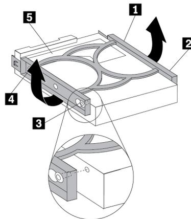
Figure 82. Installing the storage drive into the bracket
