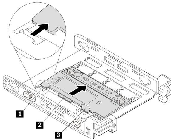
Figure 66. Pivoting the bracket
