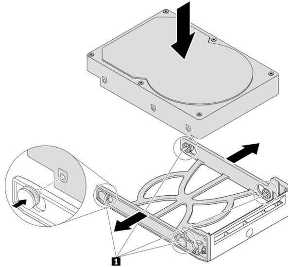
*Figure 37. Installing the 3.5-inch storage drive into the bracket*
