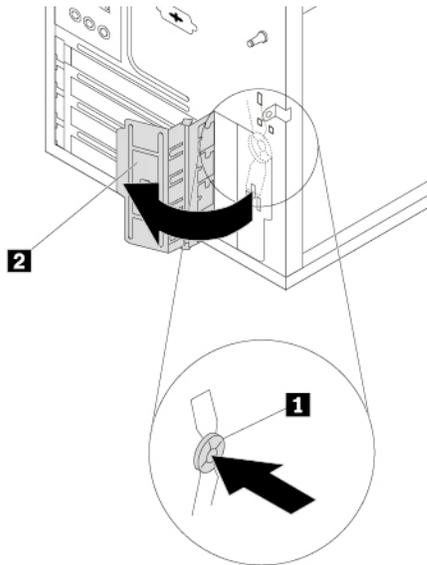
Figure 13. Opening the PCIe card latch
