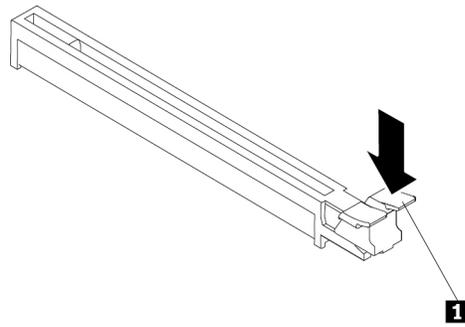
Figure 19. Disengaging the retaining latch
