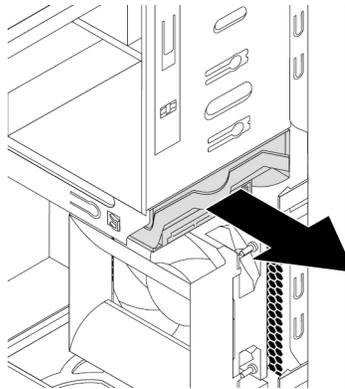
*Figure 78. Removing the primary storage drive*
