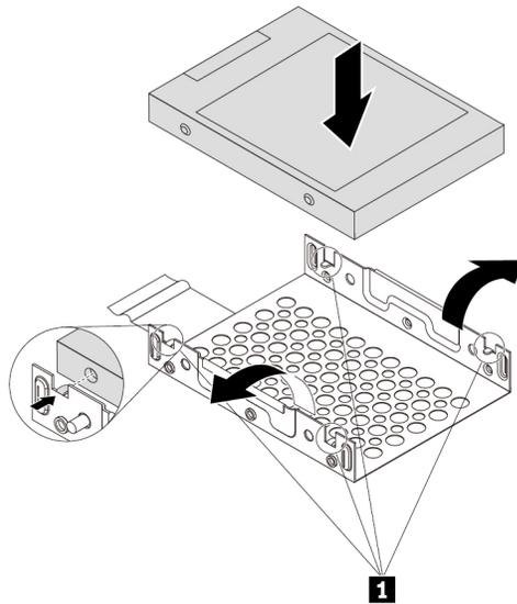
Figure 44. Installing the storage drive into the adapter
