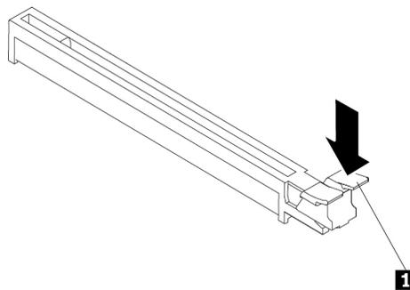
Figure 14. Disengaging the retaining latch
