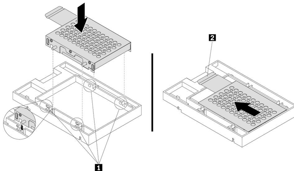
Figure 45. Installing the adapter into the converter
