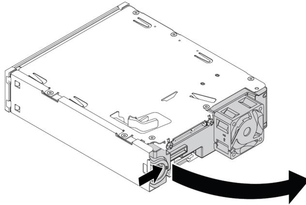
*Figure 52. Opening the rear cover of the kit*
