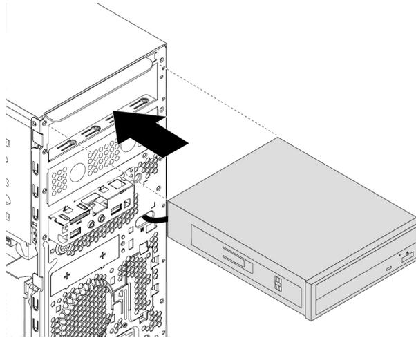
Figure 32. Installing the optical drive
