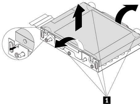
Figure 43. Removing the storage drive from the adapter
