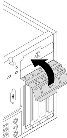
Figure 24. Closing the PCIe card latch
