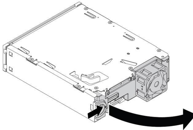
Figure 62. Opening the rear cover of the kit
