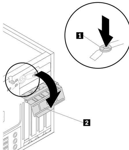
Figure 18. Opening the PCIe card latch
