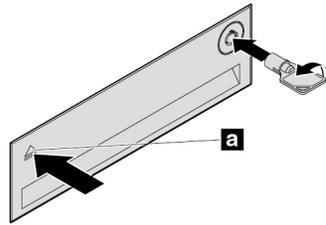
Figure 39. Opening the front-access storage enclosure cover
