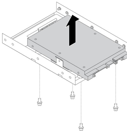
Figure 85. Removing the 2.5-inch storage drive from the storage-drive converter
