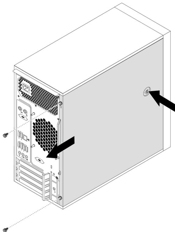
Figure 9. Removing the computer cover
