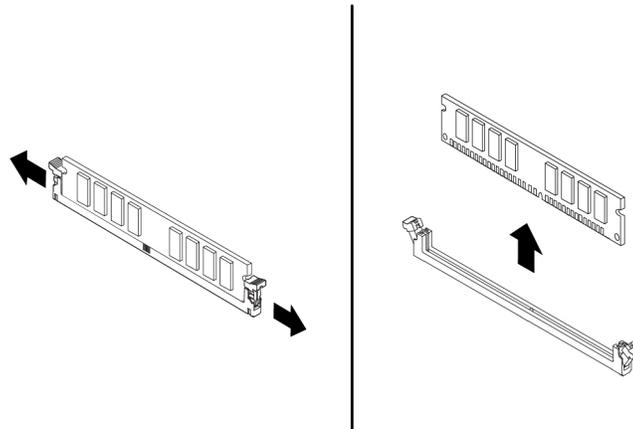
*Figure 26. Removing a memory module*
