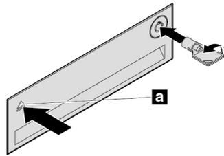
Figure 34. Opening the front-access storage enclosure cover
