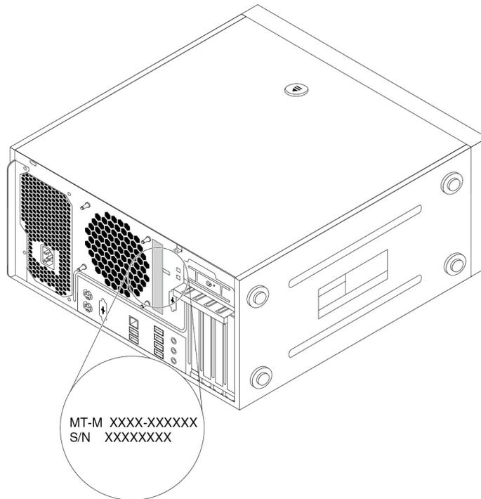
Figure 6. Machine type and model label
