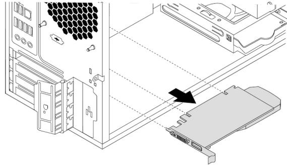
Figure 15. Removing a PCIe card
