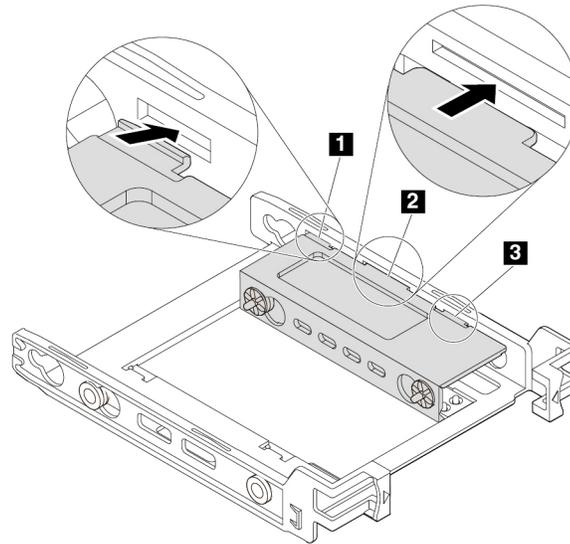
Figure 68. Inserting the tabs into the corresponding slots
