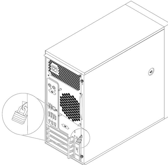
Figure 7. Installing a padlock
