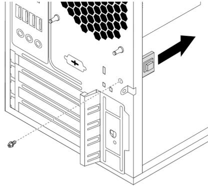
Figure 74. Removing the cover presence switch
