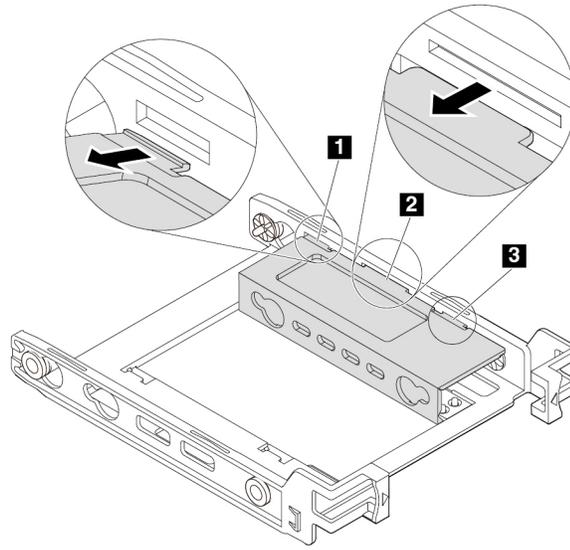
*Figure 56. Releasing tabs from the corresponding slots*
