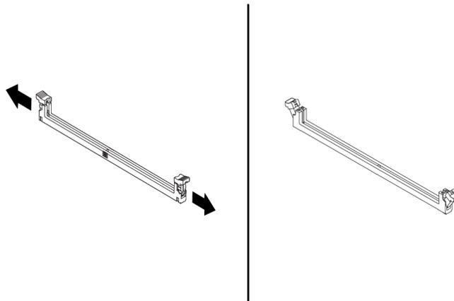
*Figure 27. Opening the retaining clips*
