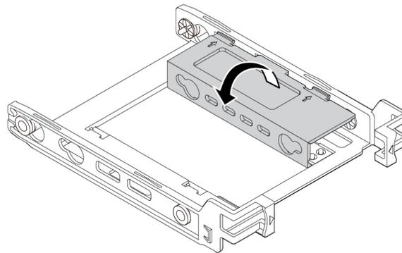
*Figure 57. Unfolding the bracket*
