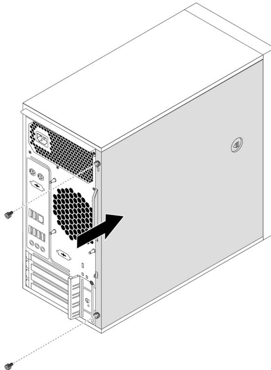
Figure 92. Reinstalling the computer cover
