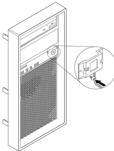
Figure 12. Installing the power button
