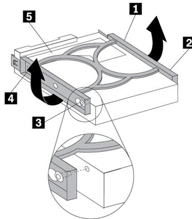
Figure 79. Installing the storage drive into the bracket
