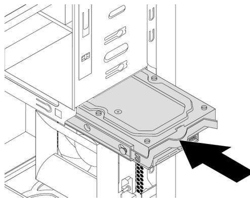
Figure 80. Installing the primary storage drive
