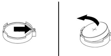
Figure 72. Removing the coin-cell battery
