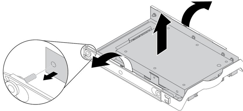
Figure 84. Removing the 2.5-inch to 3.5-inch storage-drive converter from the 3.5-inch storage-drive bracket
