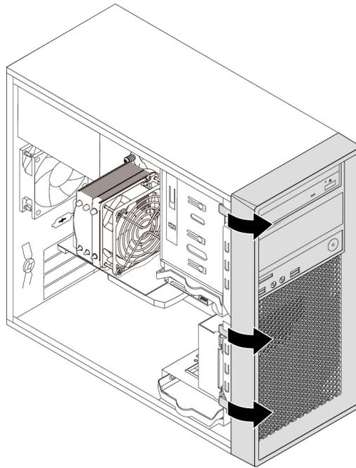
Figure 10. Removing the front bezel
