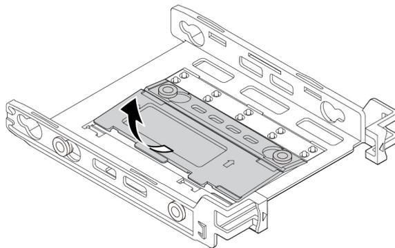
Figure 67. Folding the bracket
