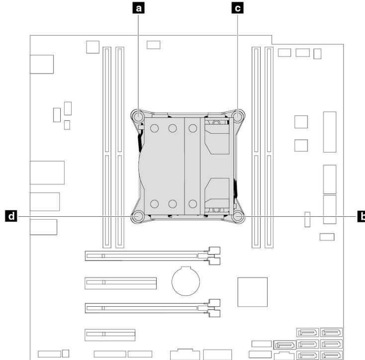
Figure 77. Removing the heat-sink-and-fan assembly
