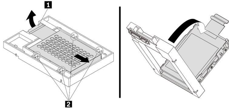
Figure 42. Removing the adapter from the converter
