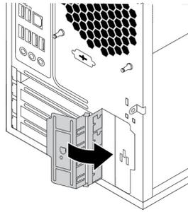
Figure 17. Closing the PCIe card latch
