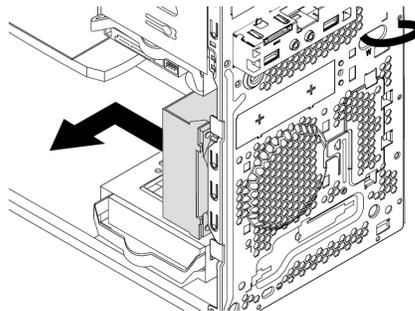
*Figure 88. Removing the front fan assembly*
