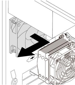
Figure 90. Removing the rear fan assembly
