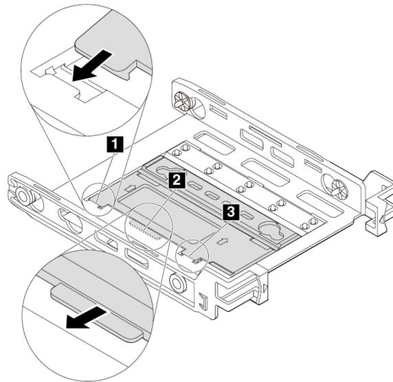
Figure 58. Inserting tabs into the corresponding slots
