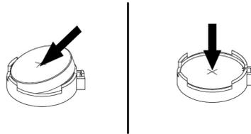
Figure 73. Installing the coin-cell battery
