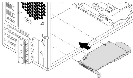
Figure 16. Installing a PCIe card
