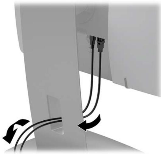
4. Connect the peripheral cables to the appropriate ports.
