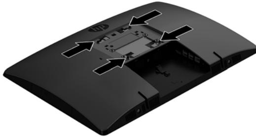
1. Press the supplied VESA trim plate onto the VESA opening until it snaps into place.
