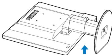
3. Release the lock of base stand then pull the base stand away from the base column.
