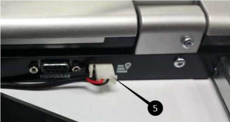
5. Connect CMA connector to back of LCD8500 1U Console as shown.
