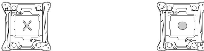
Figure 104. Applying the thermal grease to the top of the microprocessor
